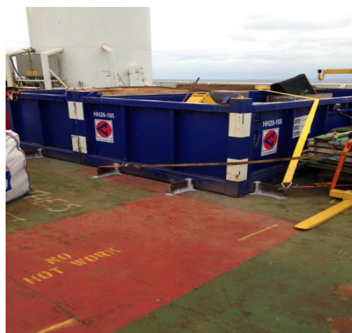
Clearly identified RED 'no hot-work' zones
